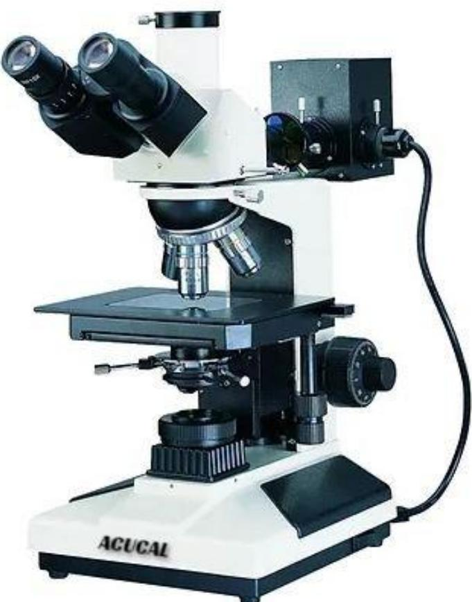
ACUMM-U2 Reflected and Transmitted Metallurgical Microscopes are suitable to observe surfaces of non-transparent object or transparent object. They are equipped with vertical illuminator and transmitted illuminator, plan achromatic objectives with long working distance (no cover glass), wide field eyepieces. They provide clear and high-contrast image, convenient control. This is ideal optical instrument for 2D Crystal Inspection.
